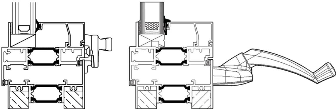
Capitol 325 ES-I Series window systems are AW-Rated thermally broken systems with a polyamide thermal break to maximize energy performance. This window series is available in multiple configurations and arrangements to meet project designs and building functionality - projected awning, hopper, casement, fixlite, and egress options available.
